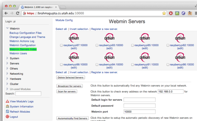
Figure 4: The webmin servers index, through which you add all other cluster nodes using a single button click or one by one in case configurations differ on each node.
